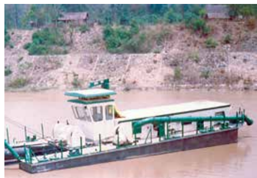
Dredging Machine for Desilting of Chatra Main Canal - SMIP
