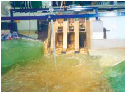
Model Testing of Dam
